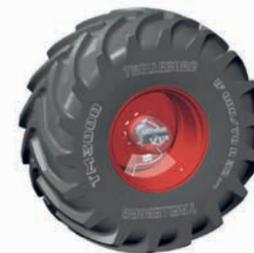
The system can automatically adjust a combine harvester's tyre pressures to reduce compaction
